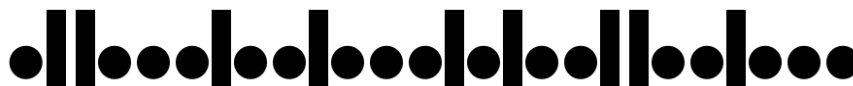
Figure 38: The Einstein model of a solid. In this diagram we have 10 oscillators. Given q dots and N - 1 separation lines, we are interested in how many choices, that is, \Omega(N, q) . Source: Wikipedia.
